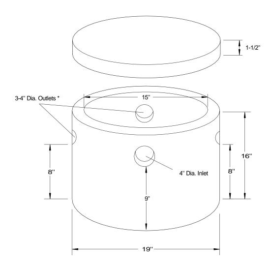
\*Outlet opposite inlet has invert height of 8-1/2". This box has no bottom; an extra lid may be used or you can pour one on site.
